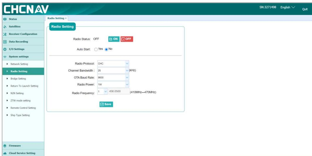
Figure 3-22 Set internal radio mode
