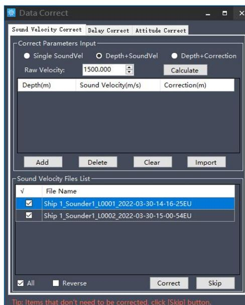
Figure 4-2 Sound velocity correction
