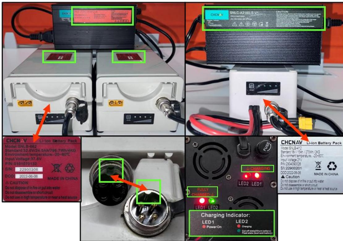
Figure 2-1 and 2-2 Battery connection during charging
