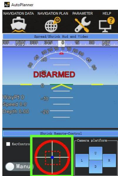
Click **[Shrink Remote-Control]**, and remotely control the USV by dragging the blue dot.
