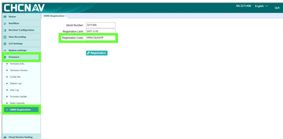
Figure 3-20 Register the receiver
