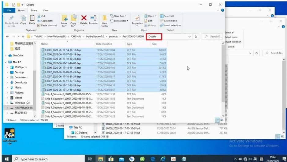
Figure 3-32 Copy dep files to the project of Hydrosurvey
