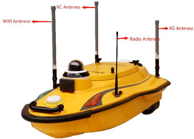
Figure 2-4 Install the accessories on the boat
